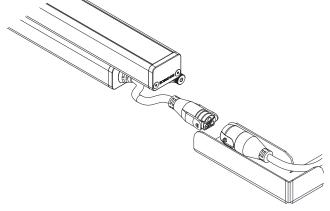
Step 6: Connect the next fixtures connector and mount to the remaining plates.
