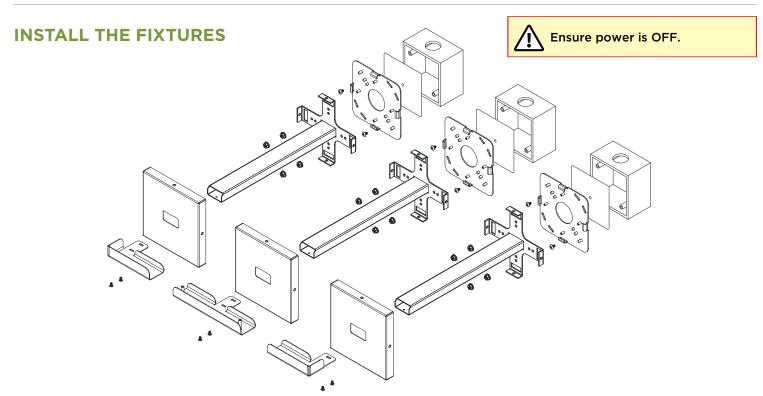
Step 1: Determine which end of the leader cable will be needed to power the first fixture in the run. Then cut off the other end and prepare the wires to be spliced. Push the cable through the center cutout on the gasket. Connect the wires to the building wires in the junction box. Punch holes for the screws on the gasket for securing the mounting plate to the junction box. Use caulking if required. Screw the mounting plate to the junction box through the gasket.
