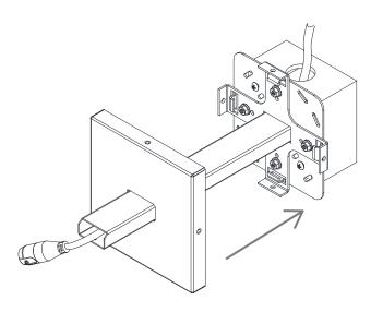
Step 4: Screw the end plates and joining plates to the arms.
