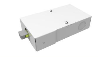
W 3.11" x H1.27" x L 5.35 ; (79mm x 32.3mm x 136mm ) APPROX LOW CARBON STEEL, 0.7mm SHEET METAL, POWDER COAT FINISH, COLOR - WHITE
