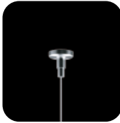
4" diameter machined power feed and 1-1/4" diameter machined non-power feed canopy. Offers minimal ceiling treatment while maintaining the ability to cover mistakes. Requires a 1/4-20 stud securely fastened to the ceiling.
