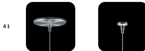
41 4" diameter machined power feed and 1-1/4" diameter machined non-power feed canopy. Offers minimal ceiling treatment while maintaining the ability to cover mistakes. Requires a 1/4-20 stud securely fastened to the ceiling. Mill, anodized, and powder coat finishes available.
