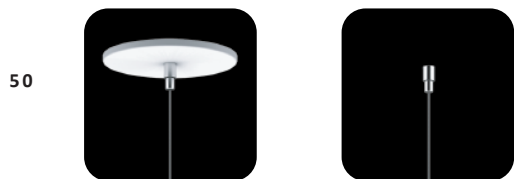
50 5" diameter power feed canopy and no canopy on the non-power feed side. Minimal aesthetic. Requires a 1/4-20 stud securely attached to ceiling. Works well with continuous runs where the power can be carried inside the fixture.
