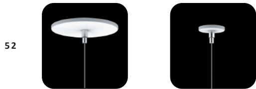
52 5" diameter power feed and 2" diameter non-power feed canopy. Offers a more minimal ceiling treatment while maintaining the ability to cover up mistakes. Requires a 1/4-20 stud securely fastened to the ceiling.
