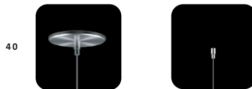
40 4" diameter machined power feed canopy and no canopy on the non-power feed side. Minimal aesthetic. Requires a 1/4-20 stud securely attached to the ceiling. Works well with continuous runs where the power can be carried inside the fixture. Mill, anodized, and powder coat finishes available.
