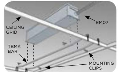
Use the TBMK mounting kit to remote mount flexed units within a grid ceiling. The EM07 is secured to the bars of the TBMK via mounting clips. The bars then mount to the T-bars of the ceiling grid. The flexible conduit of the EM07 connects to the fixture.
