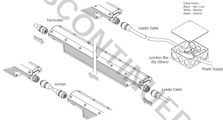
The user/installer shall provide a UL compliant junction box, strain relief and metal conduit to meet the installation requirements for the electrical connection
